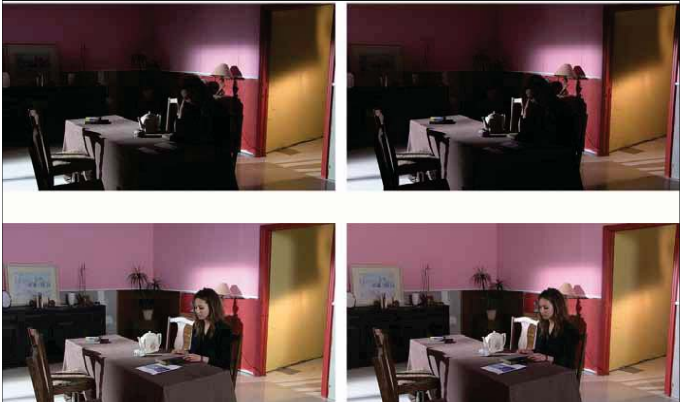
Figure 10. Use of lighting to enhance the perception of depth. Top and bottom stereo pairs are arranged for cross-eyed fusion and have the same camera parameters. The top pair has high-contrast lighting; the bottom has flat lighting. Viewers generally report that the top pair has more depth than the bottom pair.
